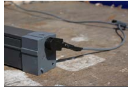
Initiated with a Detcord Loop Booster directly inserted into the end cap.
