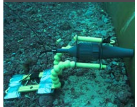
PLMEOD™ being used to detonate a US MK 25 Ground Mine. (Courtesy of the Royal Norwegian Navy).
