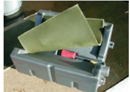
Loading QMod™ with Explosive
