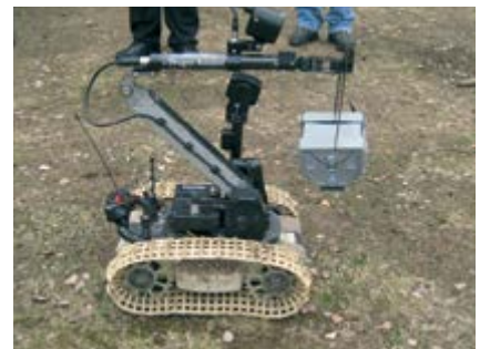
QMod™ being deployed by an ROV
